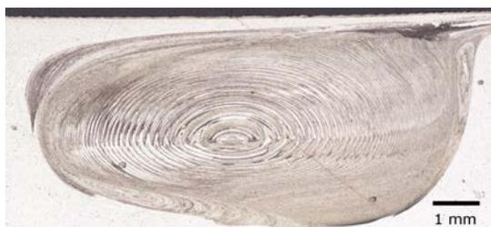
a) Tool rotational speed 500 rpm
