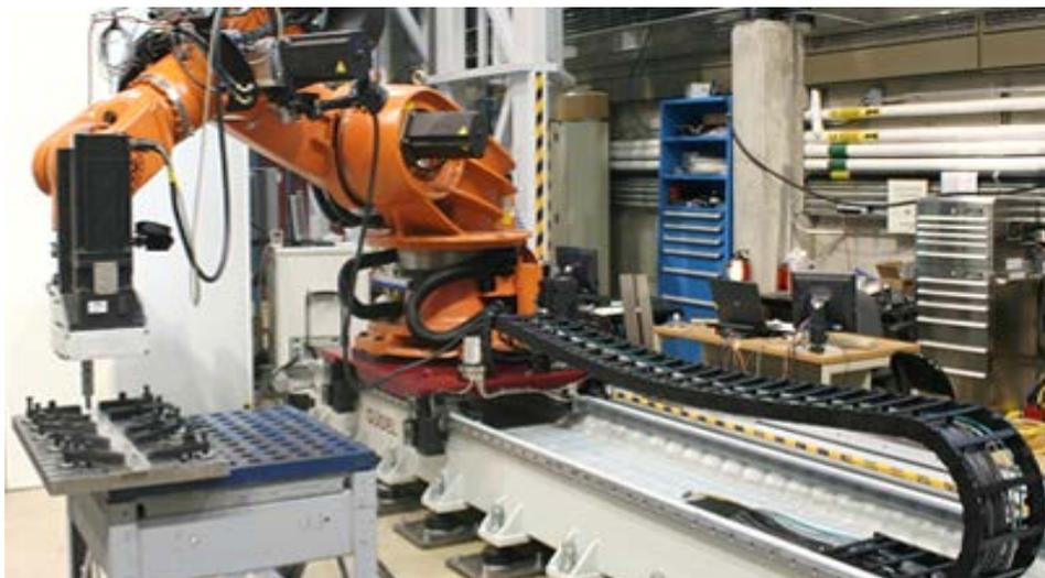
**Figure 4-2. Robotic FSW workcell incorporating a KUKA KR500-MT industrial robot mounted on a high accuracy linear unit with 5m nominal travel. In this application, the robot is performing a 1m-long weld in a planar application by maximizing contributions of rail translations during synchronized robot/rail motions.**
