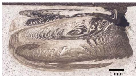
b) Tool rotational speed 500 rpm
