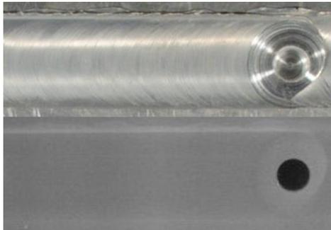
c) Tool rotational speed 500 rpm, tool travel speed 0.5 mm/s,
