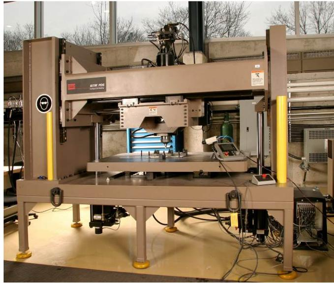
**Figure 2-4: MTS I-STIR friction stir welding system used to fabricate FSP MMCs**
